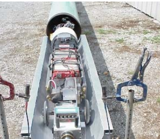
Robotic Interior Weld Coating
